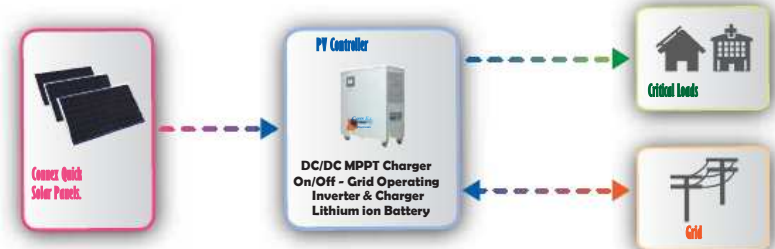
On/Off-Grid switchable Inverter and controller for 3KW system(6.63KW Lithium ion battery)
